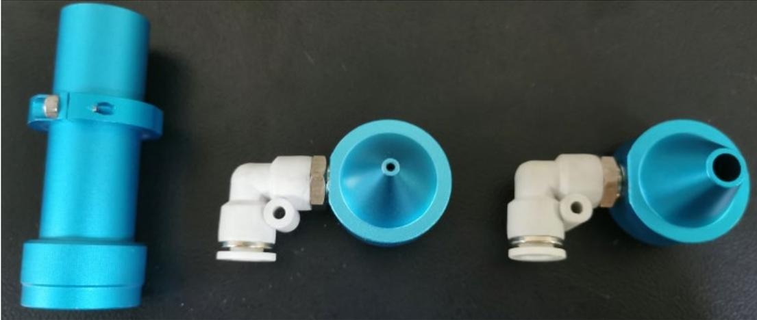
A nozzle has a very narrow outlet (approx. 2mm), which provides high air flow to blow directly on the cutting gap. This nozzle is excellently suited for cutting wood, as this prevents soot formation in the cutting gap.
