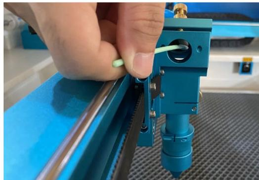
The 3<sup>rd</sup> mirror is installed on the top of the laser head.
