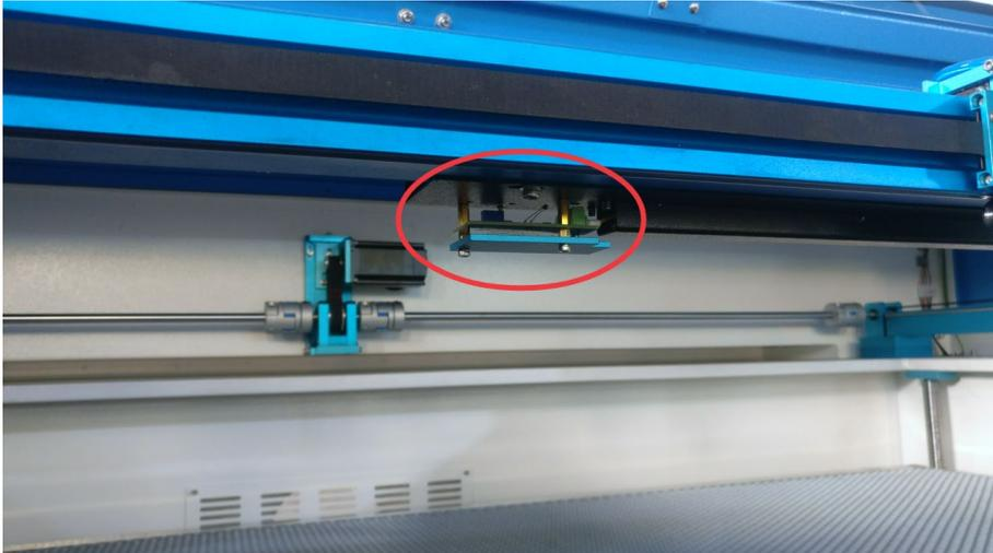
The warning sound comes from signal lamp (roughly 80dBA within 1m, 75dBA within 5m and 65dBA within 10m, the sound gets weaker as it travels).
