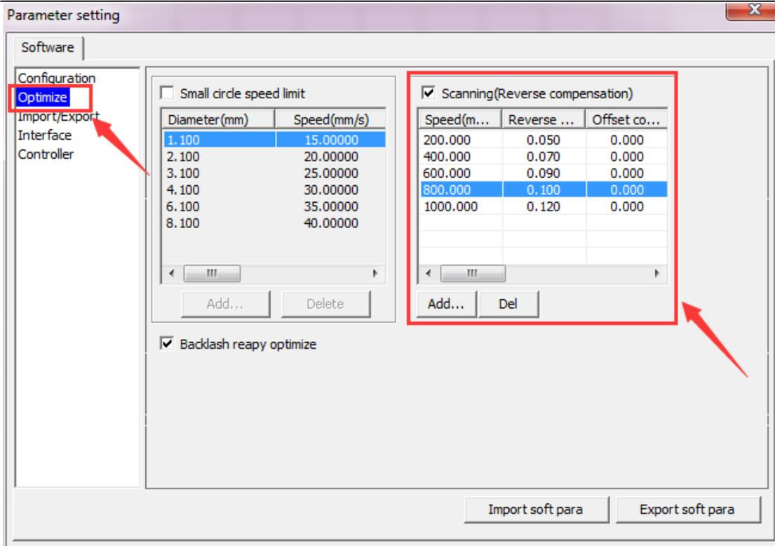
The particular values are showing with a picture in folder of laser software on the USB flash drive and on the Anodized aluminum piece that came with your machine.
