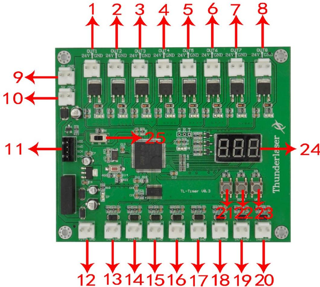
1. OUT1: Control the green light of warning light; When the machine is not at work, the warning light is in green color;
