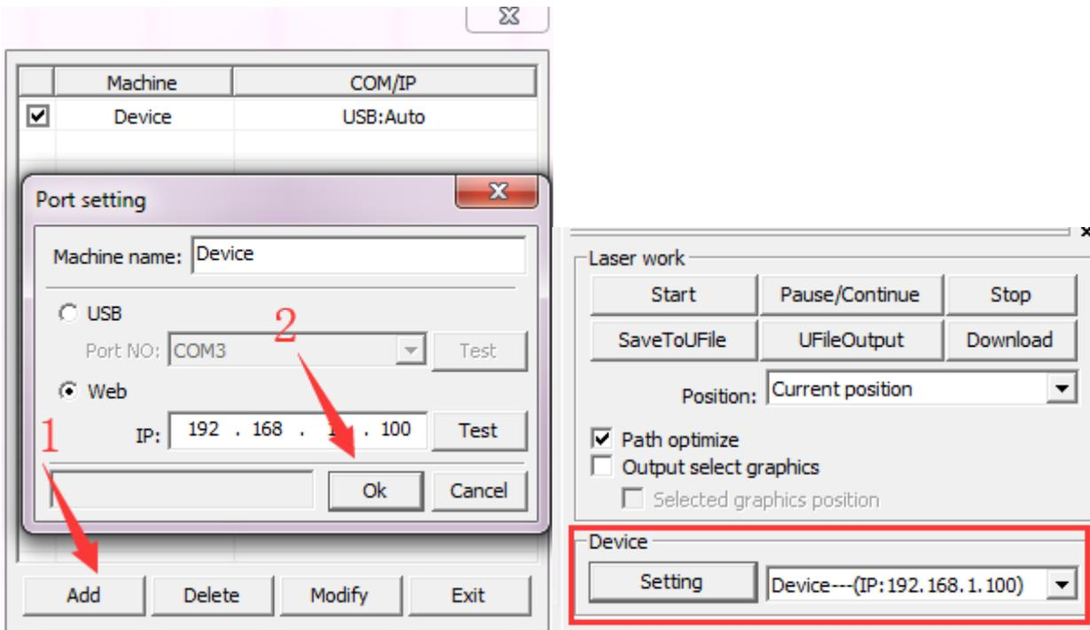
Now RDWorks communicates with your laser machine via LAN.
