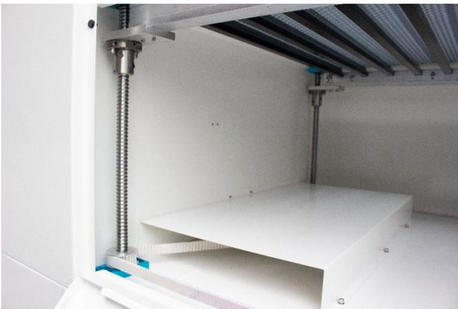
It is suggested to add lubricant oil (or Rust Preventative Grease) to the rails/screws at least every two weeks.
