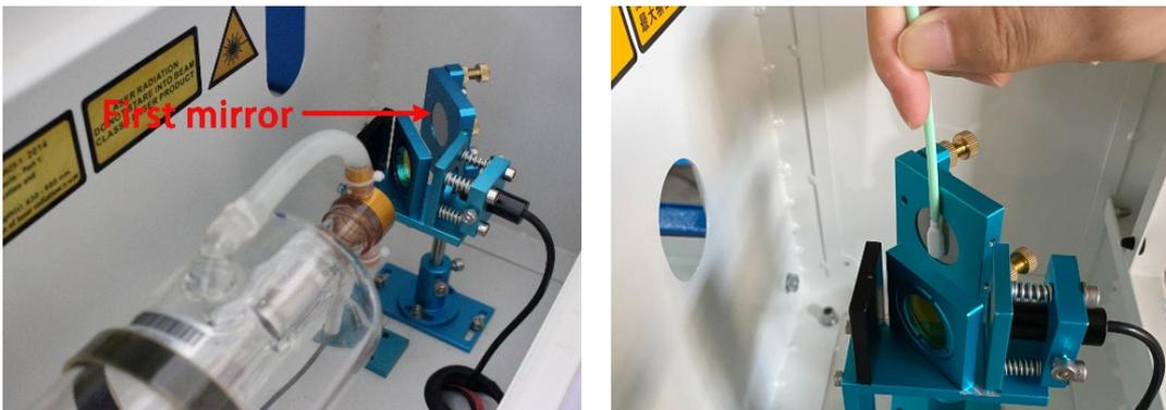
The 1<sup>st</sup> mirror is installed in the rear box of the laser tube, open it then view the right side.
