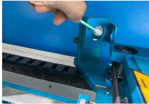
The 2<sup>nd</sup> mirror is installed on the left side of X rail.
