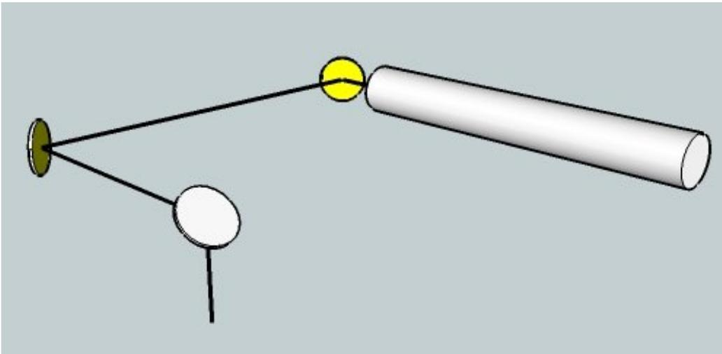
After being used for a long time, the beam path might be deflected. This will reduce the efficiency of the laser beam or even cause no laser beam. At this moment, you will need to re-adjust the beam path again.
